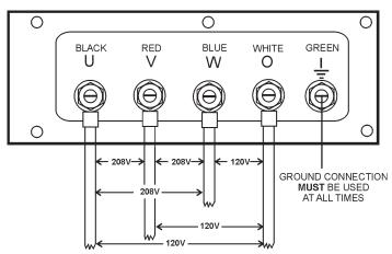
Figure 25. Output Terminal Lugs 3Ø-208/120V Connections
